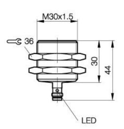
Inductive Sensors BES 516-359-G-E5-Y-S 49 M30x1.5 x 44 normally-open Sn=15mm shielded
